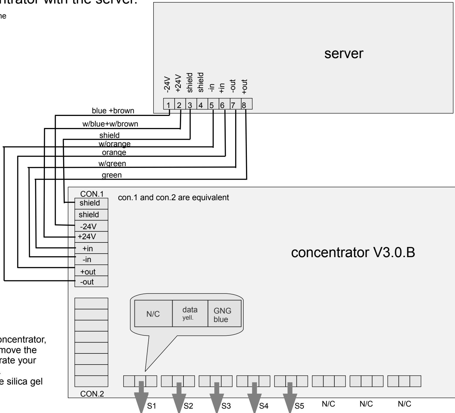
Please follow the setting of the concentrator, before the final closing of the lid, remove the packet of silica gel pouch and Integrate your free volume inside the concentrator.
