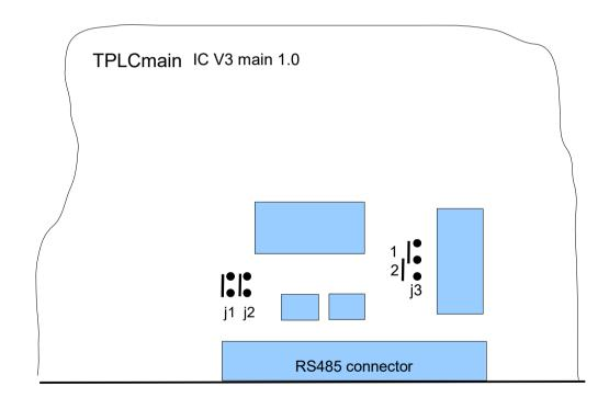
TPLC="master" in RS485 and RS232 mode j1 = on, j2 = onTPLC="slave" in RS485 and RS232 mode j1 = off, j2 = off
