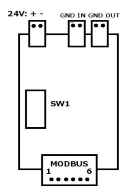
TAIO-15-1 module can provide any PLC system with one analog input and one analog output, both in the range of 0-10V and both isolated from the communication bus as well as from the input power supply.
