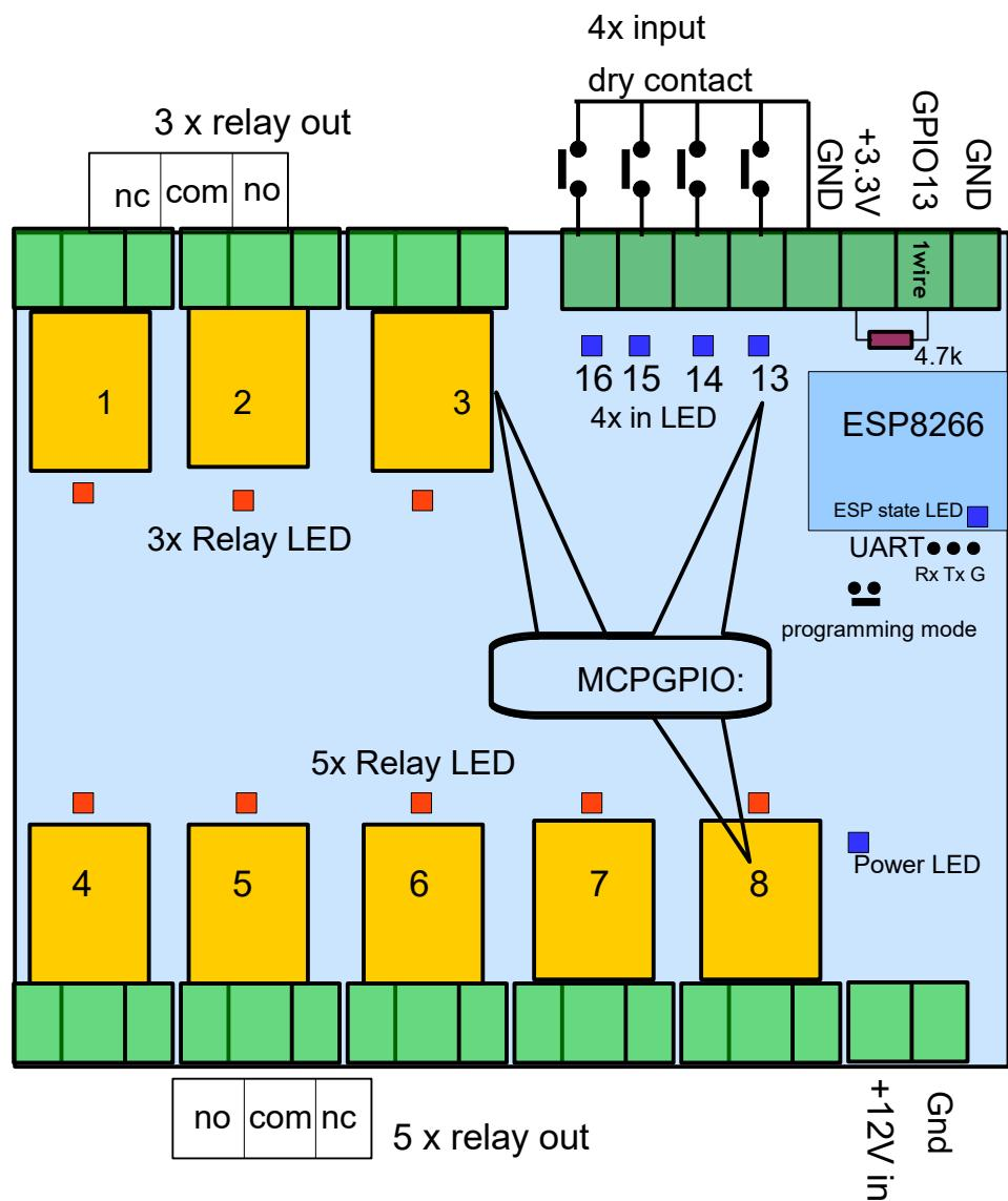
for different firmware: MCPGPIO 1 - 8 = MCPGPIO A0 - A7, MCPGPIO 9 - 16 = MCPGPIO B0 - B7
